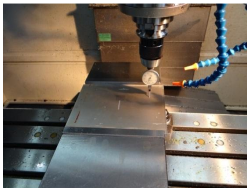
Fig. (3) Aluminum-Alloy Plates Surface-Finish Testing
