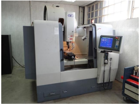
Fig. (5) The Crack-and-Grid-Implementing Computer-Controlled CNC Machine.
